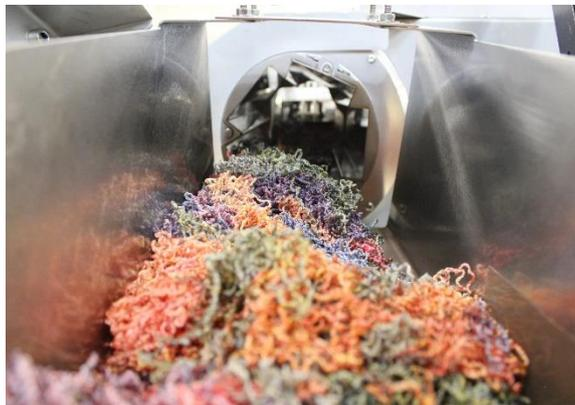
To fix the dyestuff in the fiber and lock the twist, the heat-setting lines are directly connecting to the upstream processes, thus producing a soft-touch and durable carpet yarn. Whatever the fiber type, SUPERBA is proposing the right solution:
